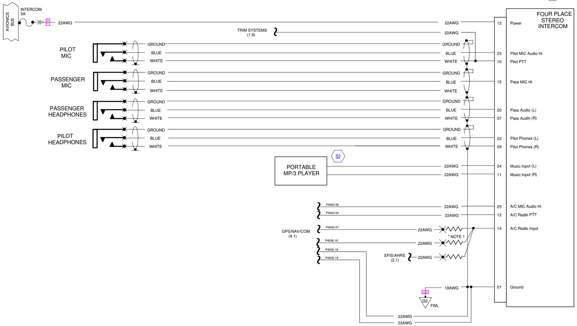
NOTE 1: This device is a 560 OHM, 1/2 WATT resistor. (Radio Shack #271-1111)
